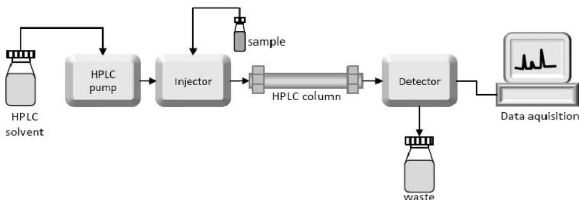
High performance liquid chromatography (HPLC) is a specialised form of column chromatography. It allows organic molecules at low concentrations to be separated from a mixture. These components can then be quantitatively analysed.
