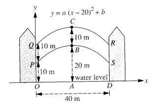
The water level is along OD. The architect introduces the x and y coordinate system for calculation purposes as shown. For example, point S has coordinates (40, 10).
