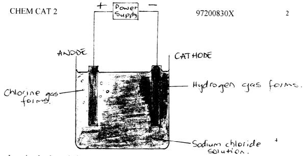
In a simple electrolytic cell, using brine as the electrolyte and unreactive electrodes, cathode will become negatively charged as the polarity of connected power supply causes electrons to migrate to this region, resulting in a reduction reaction. Chemicals present at cathode include H<sub>2</sub>O(l), Na<sup>+</sup> (aq), and Cl (aq). From electrochemical series,
