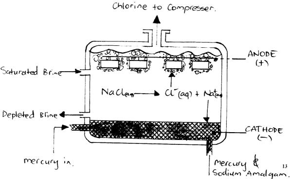
At mercury cathode, sodium cations are discharged at surface forming sodium amalgam with mercury, given by equation;
