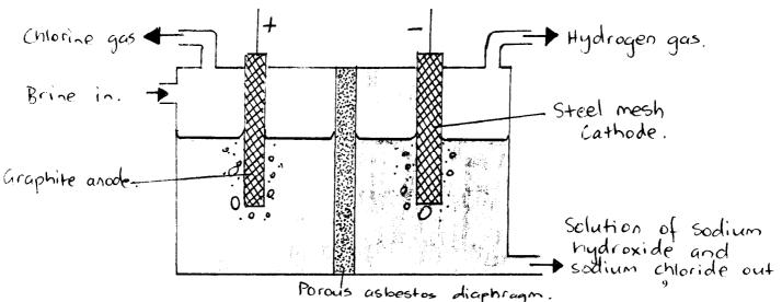
Cell is normally steel and diaphragm normally made of asbestos deposited on fine wire. Traditionally anodes made of graphite and impregnated with linseed oil or other organic materials preventing electrolytic corrosion. Ohlorine produced on graphite anodes, which are covered with incoming salt brine. Chlorine bubbles rise to top of anode and collected form chlorine pipelines connected by each cell. Chlorine gas produced contains water vapour, making it a very corrosive material.
