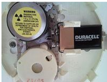
Figure 1- Americium-241 is used in smoke alarms
