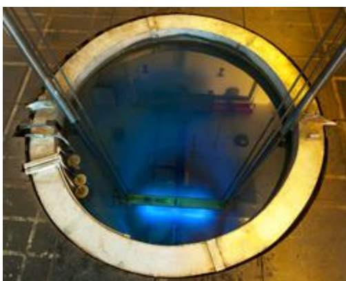
Figure 7- GATRI's Cobalt-60 Radioactive Source
